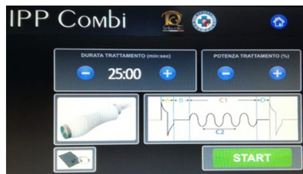
Figure 8: Treatment device for the application of the electroporation mini-current
